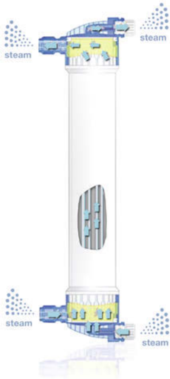
INLINE steam sterilisation process and integrity test
